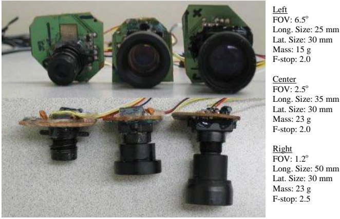
Fig. 3. Optic flow sensors with three different lens configurations: 1.2, 2.5, and 6.5 degree field-of-view. The optic flow sensors are constructed by attaching a lens to an optical mouse chip.
